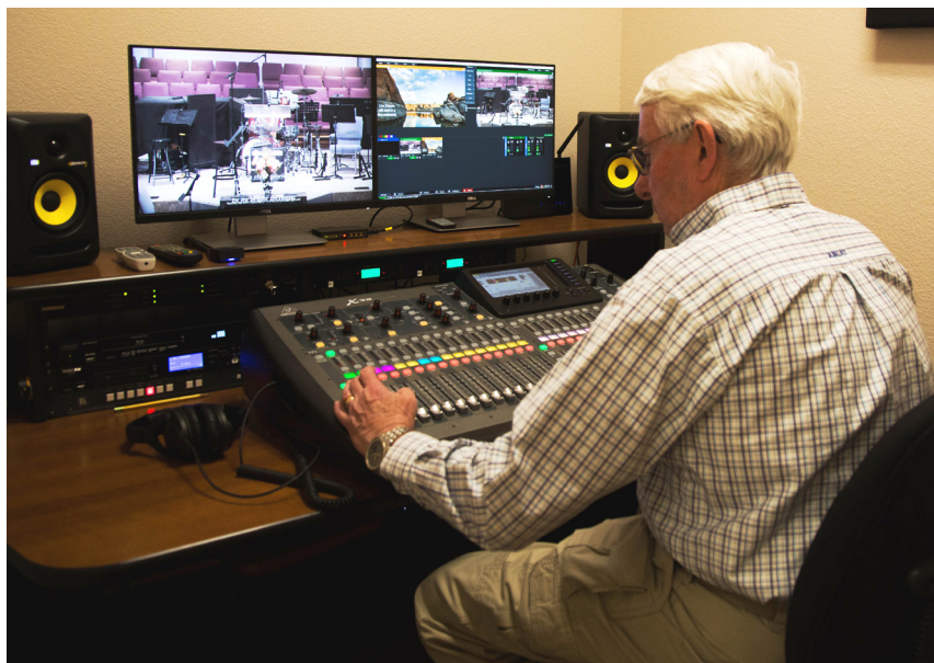
Willow Hills Baptist Church lead tech David Smith works on a Behringer X32 console in the production room, while watching the various views from the four Vaddio PTZ cameras being used in the worship space.
